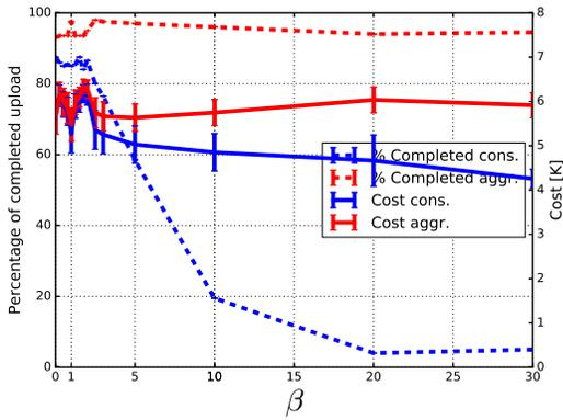
Fig. 3: Percentage of completed uploads and  $C$  versus  $\beta$  with  $S = 300s$ ,  $\alpha = 0.1$ . Trying to push a little more data than expected has positive benefits on the aggressive algorithm, but dramatic effects on the conservative algorithm
