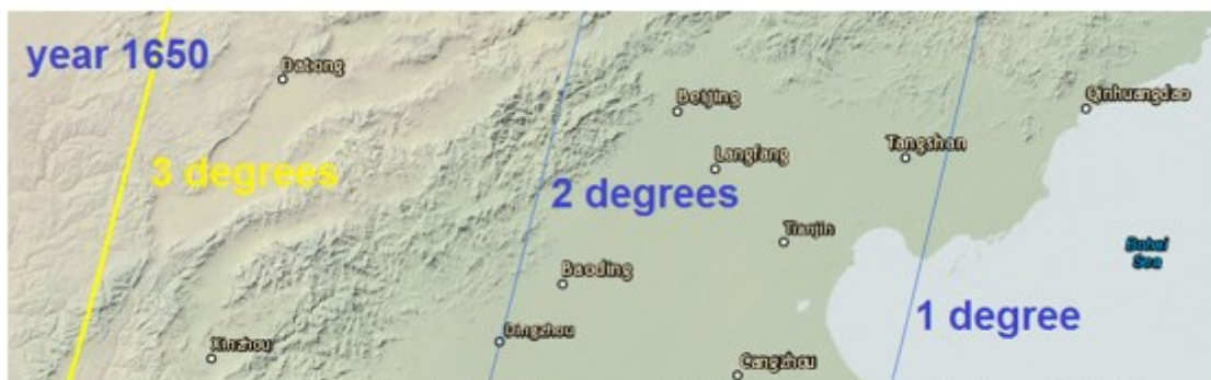
Figure 11: Again, using the interactive map of NOAA we can see that, on 1650, the magnetic declination in Beijing was between 1 and 2 degrees, negative.
