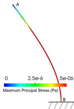
**Figure 1: explanatory example of GC deformed by applying an instantaneous fluid shear force  $\mathbf{F}_{shear}$  as obtained from CFD simulations.  $\mathbf{F}_{shear}$  is applied in A,  $\mathbf{F}_{mem}$  in B. The deformed GC structure is color-coded with the instantaneous local value of the maximum principal stress.**
