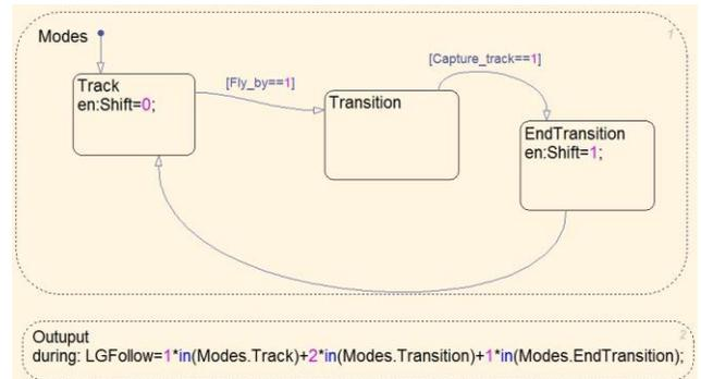
Figure 3. Flow chart of the Route Following guidance.
