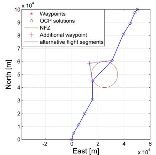
**Figure 4. Example of optimum trajectory crossing the NFZ.**
