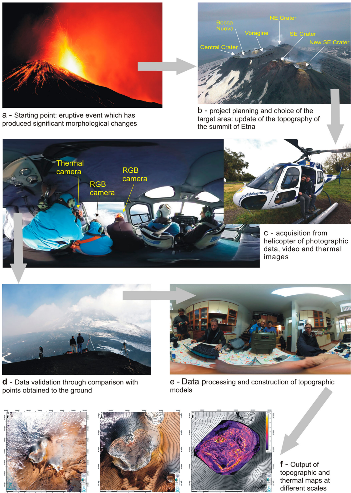
Figure 2. Flow chart illustrating the methodology followed during the construction of the topographic maps of Mount Etna summit zone.
