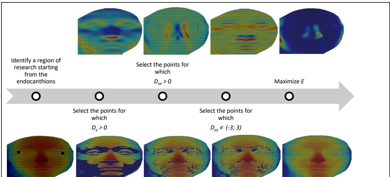
Figure 10. Process for localizing the exocanthions. The first row shows the descriptors (mapped on a face of the Bosphorus database) involved in the instruction below: (from left to right) first derivative with respect of  $y$ , second derivative with respect of  $x$ , second derivative with respect of  $y$ , coefficient  $E$ . The final row shows the gradual narrowing of the area of interest when the steps above are gradually applied. The landmarks are extracted at the final step.
