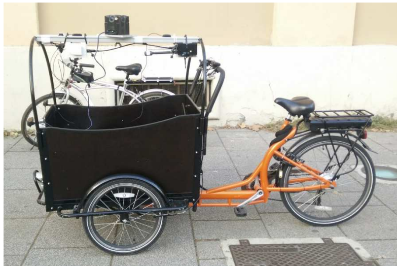
Fig. 10. Acquisition system equipped with all the imaging and environmental sensors.
