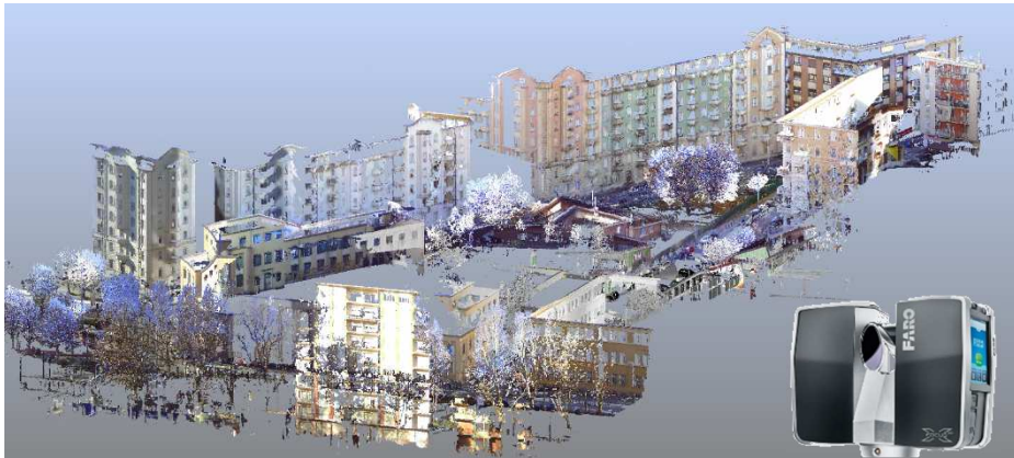
Fig. 9. Final 3D model generated through the laser scanner technology (FARO FOCUS 3D at the bottom right of the image).
