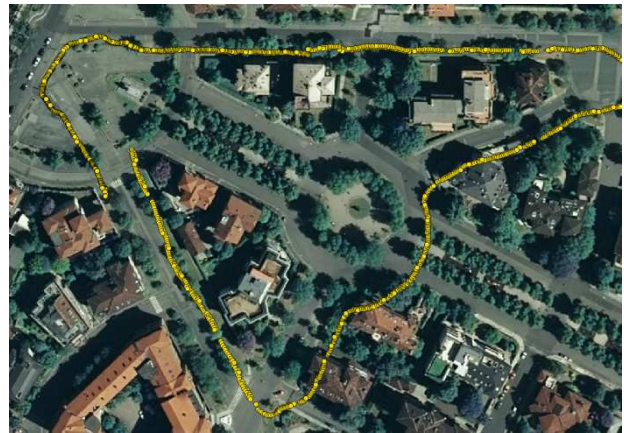
Figure 14. Camera positions estimated by Agisoft Photoscan Professional.
