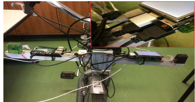
Figure 4. Bike mobile system with all sensors installed
