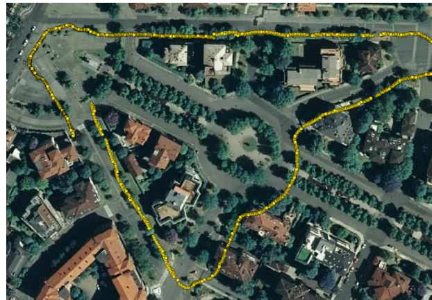
Figure 14. Camera positions estimated by Agisoft Photoscan Professional.
