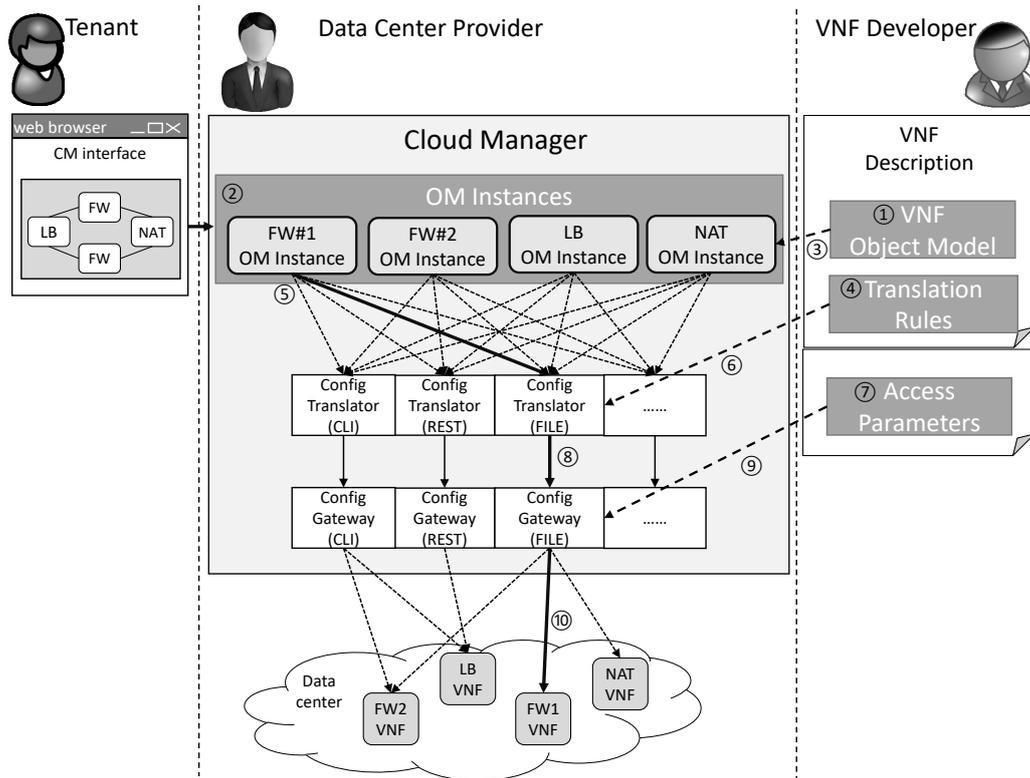
Fig. 4.3 Overview of a CM architecture for configuring VNFs.
