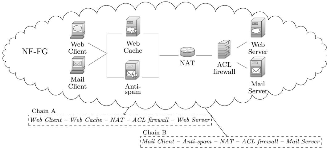
Fig. 3.4 An example of Network Function-Forwarding Graph.
