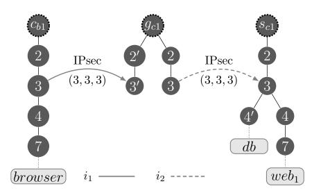
Fig. 6.13 Graphical representation of a monitorability anomaly.
