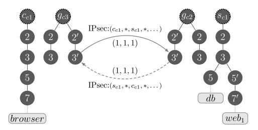
Fig. 6.2 Graphical representation of a site-to-site communication.
