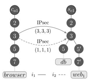
Fig. 6.11 Graphical representation of an inclusion anomaly.
