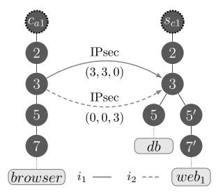
Fig. 6.6 Graphical representation of shadowing and exception anomalies.
