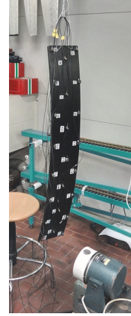
FIGURE 4: The leaf spring component: the experimental configuration with 23 accelerometers.
