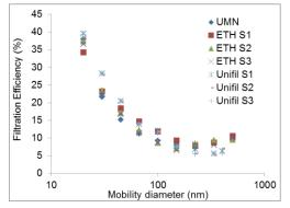
The figure on the left shows some filtration efficiency data referring to different wire mesh samples and laboratories. The data were measured at 5 cm/s face velocity.
