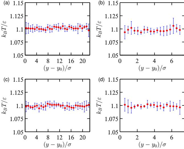
FIG. 8. Temperature profile ( $k_B T / \epsilon$ ) of the LJ fluid along the channel width: (a)  $h = 21.44\sigma$  and  $\epsilon_w = \epsilon$ ; (b)  $h = 6.43\sigma$  and  $\epsilon_w = \epsilon$ ; (c)  $h = 21.44\sigma$  and  $\epsilon_w = 0.2\epsilon$ ; (d)  $h = 6.43\sigma$  and  $\epsilon_w = 0.2\epsilon$ .
