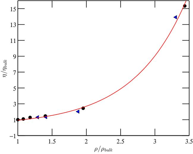
FIG. 11. Normalised density ( $\rho/\rho_{bulk}$ ) vs. normalised viscosity ( $\eta/\eta_{bulk}$ ) at the density peaks for channel widths  $h = 21.44\sigma$  (black circles) and  $h = 6.43\sigma$  (blue triangles). The red solid line is a fit to Eq. (C1), with fitting parameters  $a = 0.19$ ,  $b = 1.28$  and  $c = 0.31$  ( $R^2 = 0.9974$ ).
