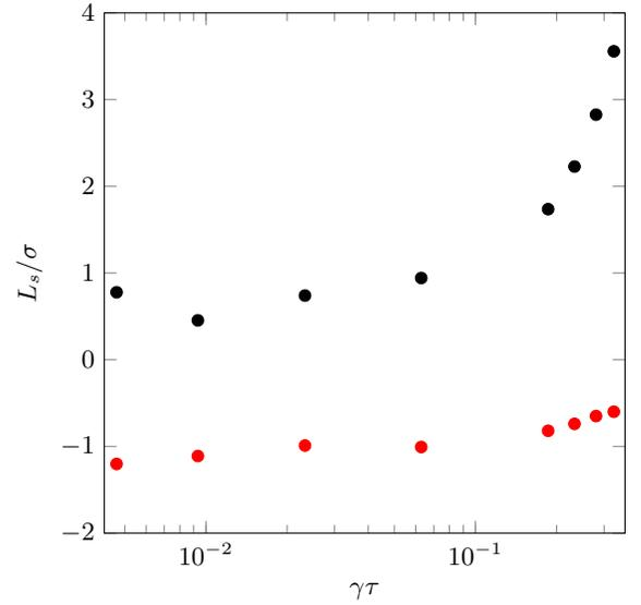
FIG. 9. Slip length ( $L_s / \sigma$ ) as a function of the shear rate ( $\gamma\tau$ ). The nanochannel width is  $h = 21.44\sigma$ ; black circles and red squares correspond to  $\epsilon_w = 0.2\epsilon$  and  $\epsilon_w = \epsilon$  respectively.
