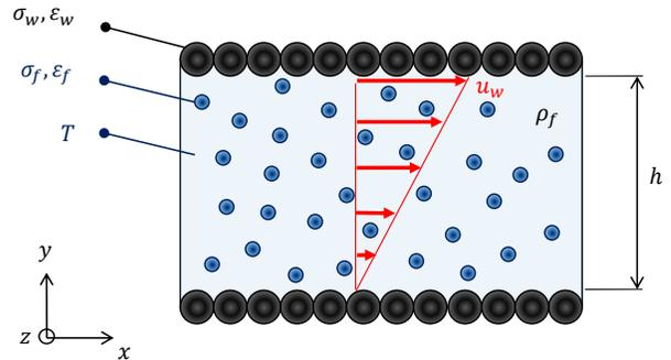
FIG. 1. Sketch of the atomistic view of a Couette flow of a LJ fluid at temperature  $T$  through a channel of width  $h$ . The top wall is sheared with velocity  $u_w$ . The velocity profile of the flow is shown by the red arrows. The fluid and wall LJ parameters are  $\epsilon_f, \sigma_f$  and  $\epsilon_w, \sigma_w$ , respectively.
