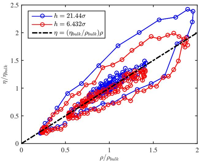
FIG. 7. Viscosity vs. density for two channel widths for hydrophilic substrates and comparison with linear relationship  $\eta = (\eta_{bulk}/\rho_{bulk})\rho$  for all but the first particle layers nearest the walls. The data has been averaged for each channel width exploiting the spatial symmetry in the  $y$  direction. The linear relationship requires knowledge of only the bulk values of density and viscosity, and achieves an  $R^2 = 0.83$  fit to the data.
