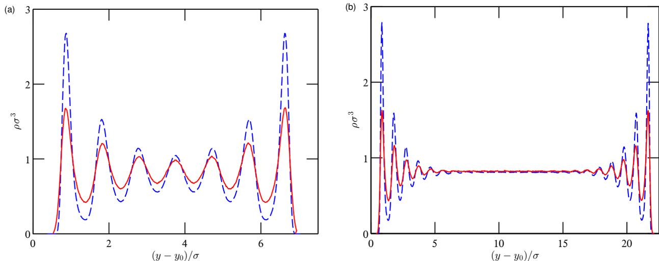
FIG. 2. Fluid density profiles,  $\rho$ , across the nanochannels of width (a)  $h = 6.43\sigma$  and (b)  $h = 21.44\sigma$ . Blue dashed and red solid curves correspond to the hydrophilic ( $\varepsilon_w = 1.0\varepsilon$ ) and hydrophobic ( $\varepsilon_w = 0.2\varepsilon$ ) walls, respectively.
