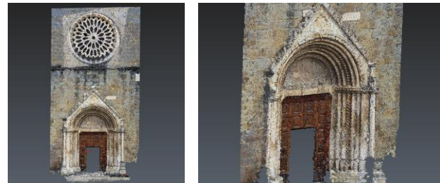
Figure 17. First test of point cloud generation of the portal before the earthquakes
