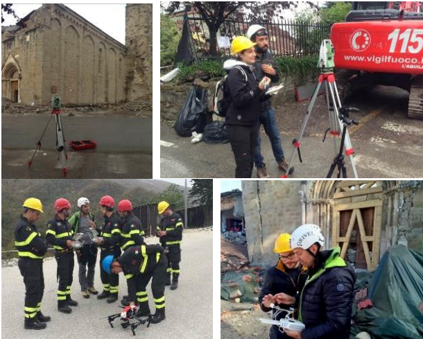
Figure 4. Survey operation in the area of Sant'Agostino; The RPAS group of the Firefighters with the INSPIRE 1; Remote control of the UAV during the image acquisition phase.
