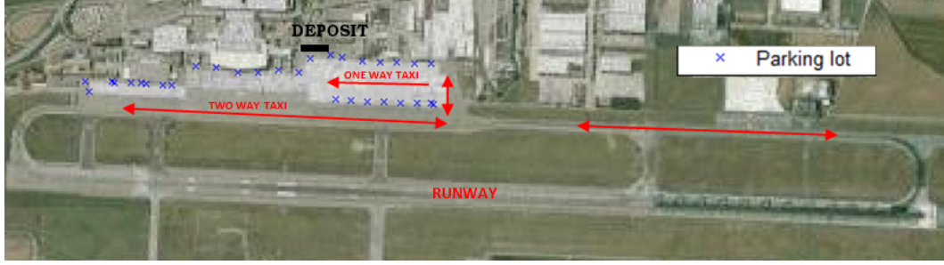
Fig. 4.1 Turin airport layout with indication of the taxiway direction and of the depot. Credits: Pictures 2015 DigitalGlobe, Map data ©2015 Google
