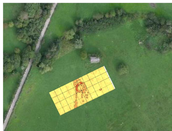
Figure 5. (Above) GPR profiles planning, topographically located onto the orthomosaic. (Below) Superimposition of time-slice at 0.7 m of depth on orthomosaic, with main anomalies derived from geophysical prospections highlighted.
