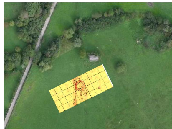
Figure 5. (Above) GPR profiles planning, topographically located onto the orthomosaic. (Below) Superimposition of timeslice at 0.7 m of depth on orthomosaic, with main anomalies derived from geophysical prospections highlighted.
