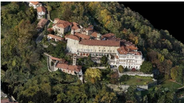
Figure 9. Two different bird eye views of the processed dense cloud. (18 milion points)
