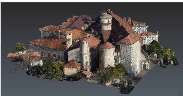
Figure 10. Other two views of an excerpt of the colored cloud; 0.026 m RMSE on GCP shows a good ability to represent the dense edification.
