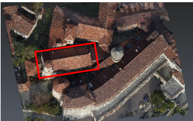
Figure 9. Two different bird eye views of the processed dense cloud. (18 milion points)
