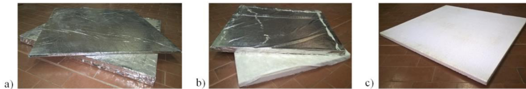
Fig. 2. Samples: (a) VIP 10 and 30 mm thick; (b) punctured VIP and VIP core material; (c) XPS.
