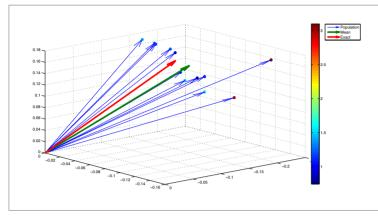
**5** Matlab\* reconstruction of magnetic field measurements: sample mean and sensor dispersion, evaluated by means of Malanobis distance (software Supervision module)
