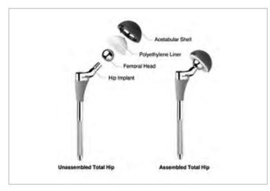
**1** *HIP prosthesis.* Components of a hip prosthesis. Source: http://www.zimmer.com/ctl?op =global&action=1&id=8140&template=PC
