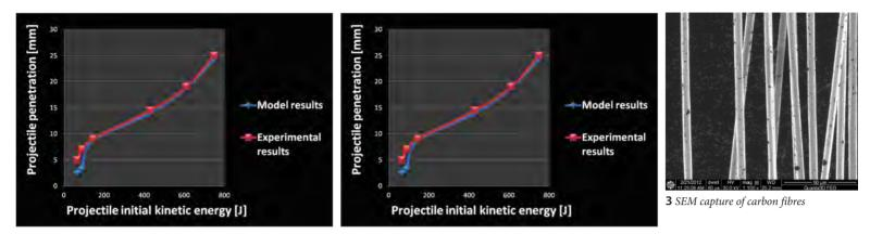
**1** Projectile penetration vs. initial kinetic energy
