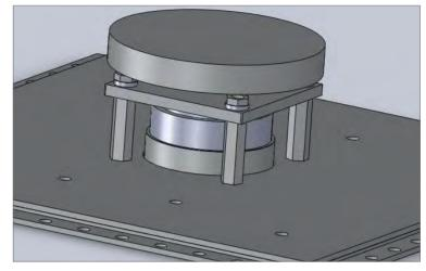
**8** *Simulation representation of the wheel mechanical support, designed by ARAM-AOCS team A*
