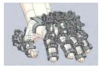
**5** The overall exoskeleton structure
