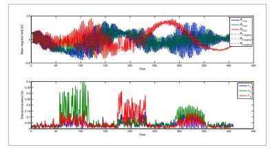
**6** *Matlab\** sensor performance evaluation and hardware failure identification (software Supervision module)
