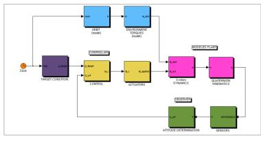
**1** *Schematic of the Dynamic Attitude and Control simulation architecture built and used by the team to test the software algorithm, using Simulink*<sup>\*</sup>
