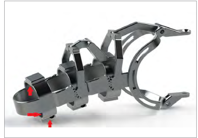
8 Prototype finger with sensors' positions indicated
