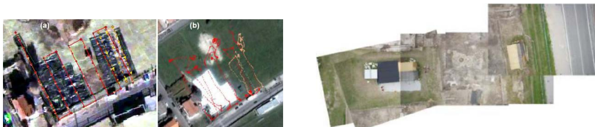
Fig.2: Left: Planned (a) and realized flight (b) with a drone. Right: sample of an image mosaicking
