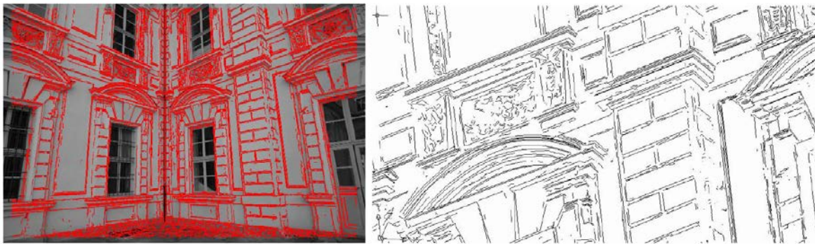
Fig. 8: Automatic extraction of breaklines from point clouds and digital image integration
