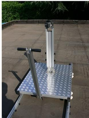
Figure 4.5 A detail of the dolly platform and of the linear slider that constraints the motion of the platform
