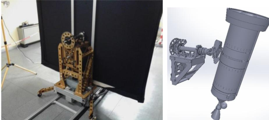
Figure 4.3 Mechanism for rotating the mock-up around a fixed axis in the inertial space. In the left image, one of the extremes of the visible cylindrical arm is hinged to a fixed platform welded to the base. The other extreme is hidden by a black panel. The right image shows the connection to the mock-up
