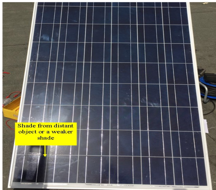
Fig. 2.11 Partial shading caused by a distant object.
