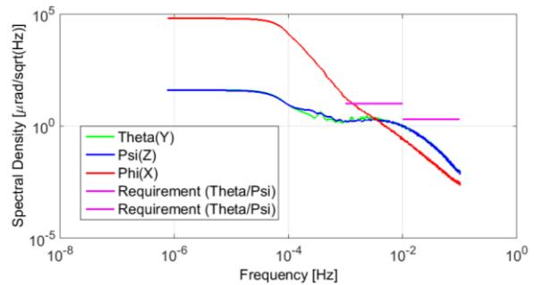
Fig. 9. Simulated PSD of the attitude 2D pointing
