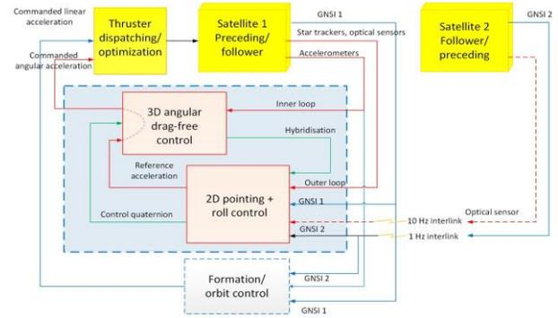
Fig. 4. Overall scheme of the attitude control unit.
