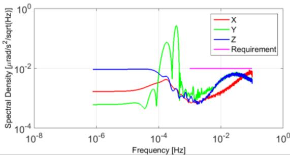
Fig. 6. Simulated PSD of the angular non-gravitational residuals
