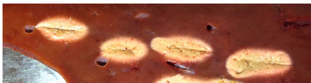
Fig. 14. Sequence of ablations keeping the energy constant at 300J; from left to right: 2W, repetition of 2W, 3W and 4W.
