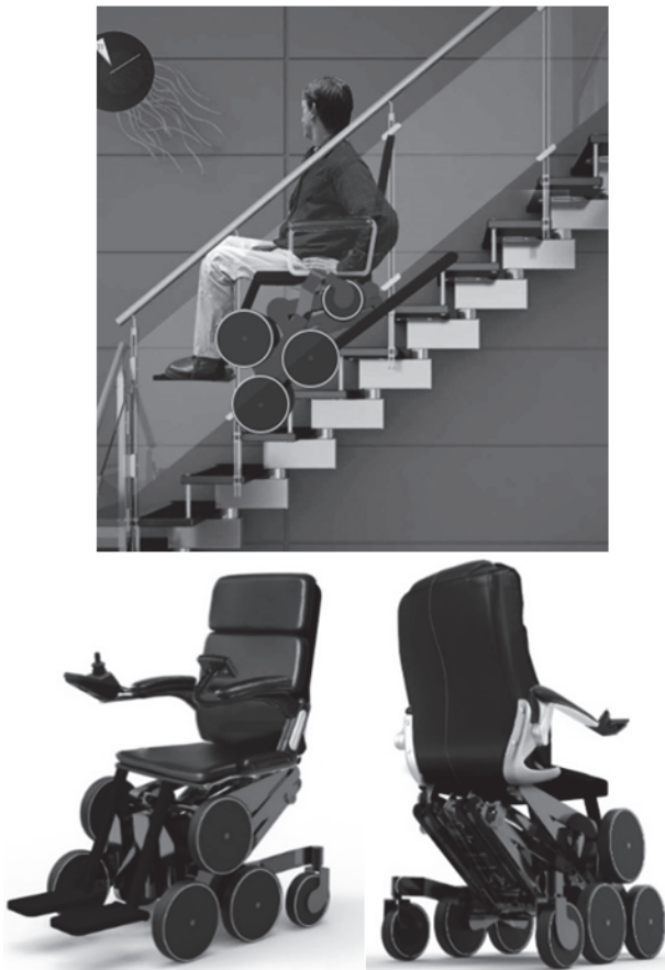
Fig. 20. Representation of a possible prototype for the proposed wheelchair.
