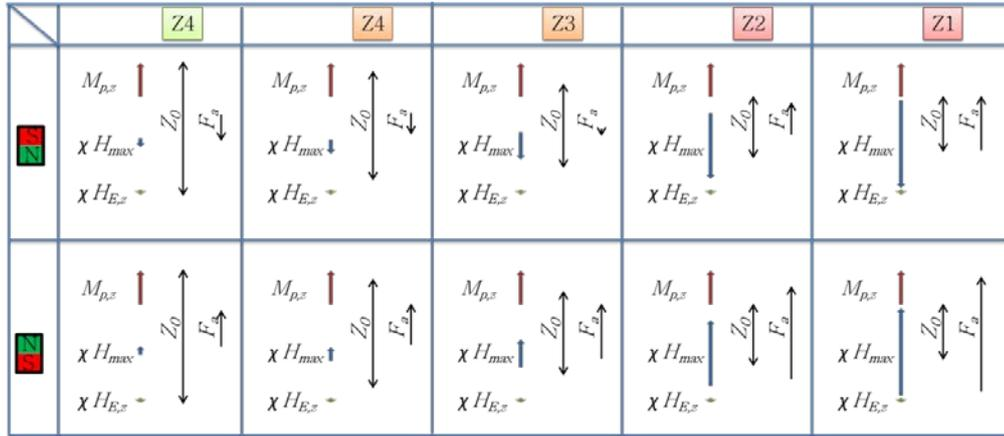
Fig. 2.29 Graphical representation of vectors of the induced magnetization  $\chi H_{max}$  and  $\chi H_{E,z}$  by the permanent magnet ( $H_{max}$ ) and by the earth's field strength ( $H_{E,z} = 50 \text{ A/m} \approx 0.6 \text{ Oe}$ ), respectively, the permanent magnetization of the sample ( $M_{p,z}$ ), and the weight,  $F_z$ , feel by the balance as function the five different distances from the permanent magnet, and its two orientations: [S|N] and [N|S].
