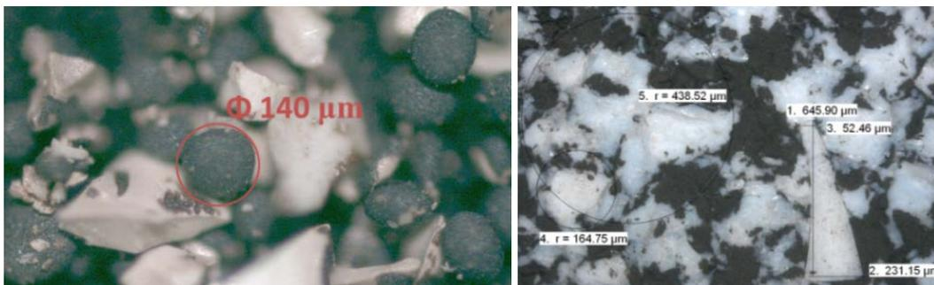
Fig. 2.13 Optical micrographs of (left)  $\text{CoFe}_2\text{O}_4$  (black) and amorphous  $\text{SiO}_2$  (white) powders mixed in a weight ratio of 80:20, respectively, by 3D turbula mixing, and (right) surface of the green sample.
