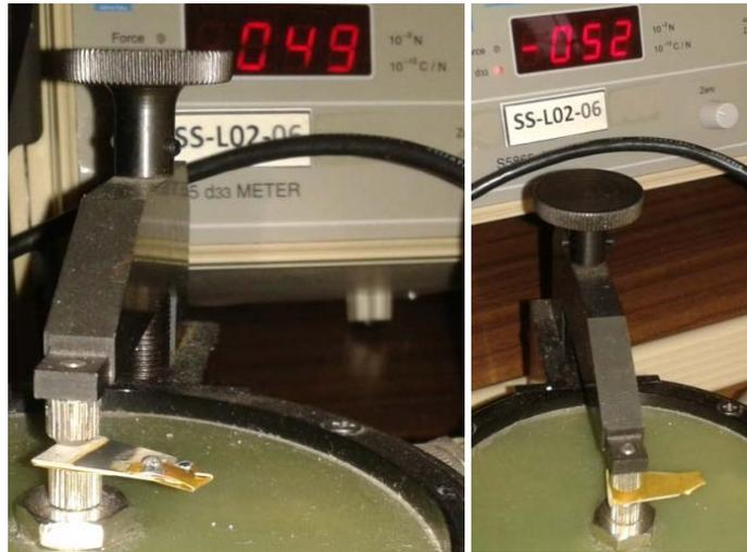
Fig. 3.40 The device is formed by top silver electrode, PZTN layer, cobalt ferrite layer, bottom silver layer, alumina substrate, brass foil electrically contacted to the bottom silver layer.
