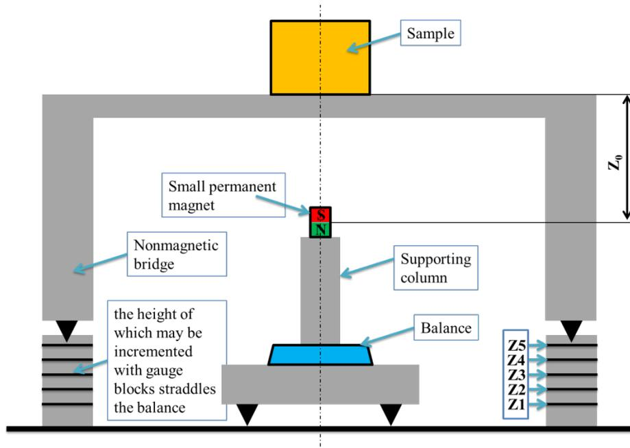
Fig. 2.28 Schematic view of the susceptometer. The sample is placed on the bridge, directly above the magnet at a distance of  $Z_0$ . In the case of Sartorius susceptometer YSZ 02C, the distance  $Z_0$  is equal to 18 mm, 20 mm, 27 mm, 35 mm, and 43 mm for Z1, Z2, Z3, Z4, and Z5, respectively.
