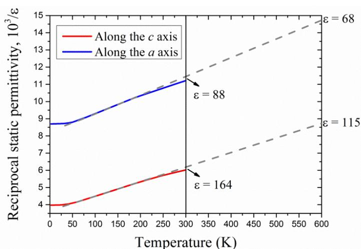
Fig. 3.28 Temperature dependences of the reciprocal static dielectric constants along  $a$  and  $c$  axes of  $\text{TiO}_2$  rutile. The solid lines were measured by G. A. Samara P. S. Peercy [106]. The dashed lines depict was calculated through the Curie-Weiss law.
