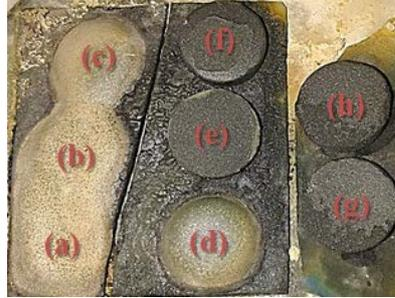
Fig. 3.29 PZTN-CF samples after thermal treatment at 1200 °C for 2 h. The samples labelled with (a, b), (c, d), (e, f), and (g, h) are characterized by cobalt ferrite molar fraction of 0.26, 0.32, 0.58, and 0.81, respectively.
