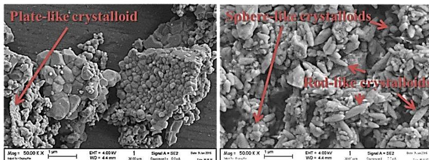
Fig. 2.4 Cobalt ferrite powders with low fractal dimension and low specific surface area synthesized by sol-gel method and post-fired at 700 °C for 3 h.
