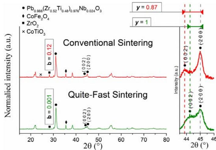
Fig. 3.32 XRD patterns of sintered PZTN-CF ( $x = 26$ ) composites.
