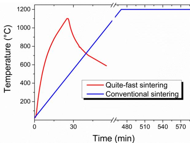
Fig. 2.16 Heating profile of quite-fast sintering (red curve,  $T_{\max} = 1100$  °C) and conventional sintering (blue curve,  $T_{\max} = 1200$  °C).
