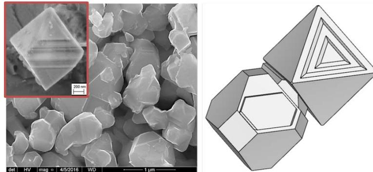
Fig. 2.2  $\text{CoFe}_2\text{O}_4$  powders calcined at 1050 °C for 4 h (left), and a graphical representation of some possible octahedron shapes build up starting from the crystal lattice refined from X-ray diffraction data (right).
