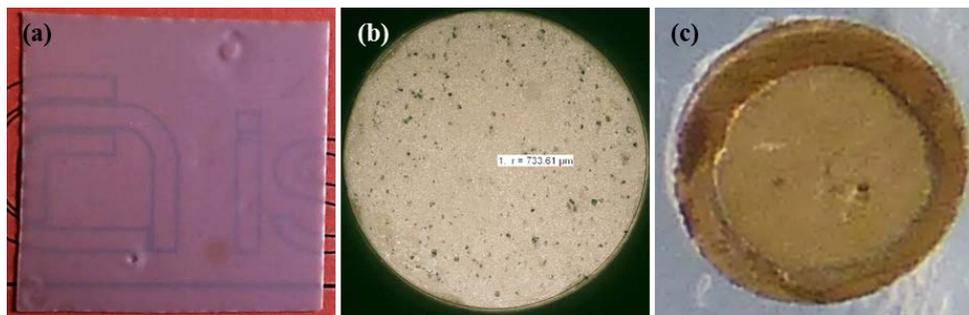
Fig. 2.22 (a) Sintered tape of Nb-doped lead zirconate titanate (PZTN) characterized by a thickness of  $t = 70 \mu\text{m}$ ; (b) PZTN disk ( $\phi 1.5 \text{ mm}$ ) obtained from the tape; (c) PZTN disk sputtered with gold, poled, and glue on a brass disk ( $\phi 2 \text{ mm}$ ,  $t = 0.3 \text{ mm}$ ).
