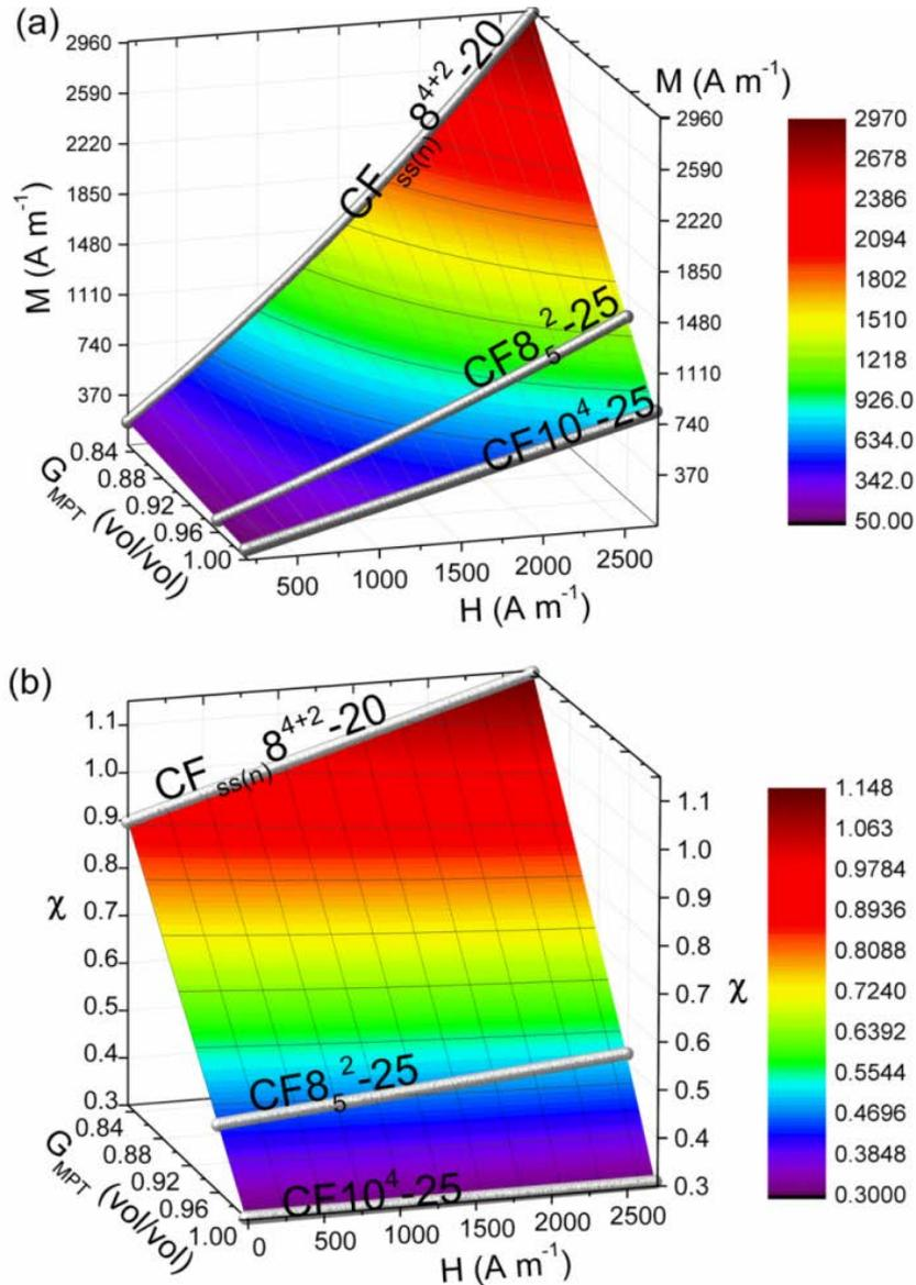
Fig. 3.14 Plot of (a) magnetization ( $M = \chi H$ ) and (b) volume magnetic susceptibility ( $\chi = \chi_i + \alpha H$ ) as a function of magnetic field strength ( $H$ ), and multiparallel-twinned grains volume fraction ( $G_{MPT}$ ).
