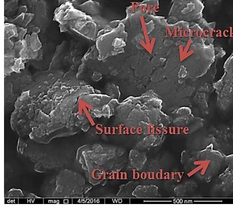
Fig. 2.11 Defects can reduce the resistance of the particles.
