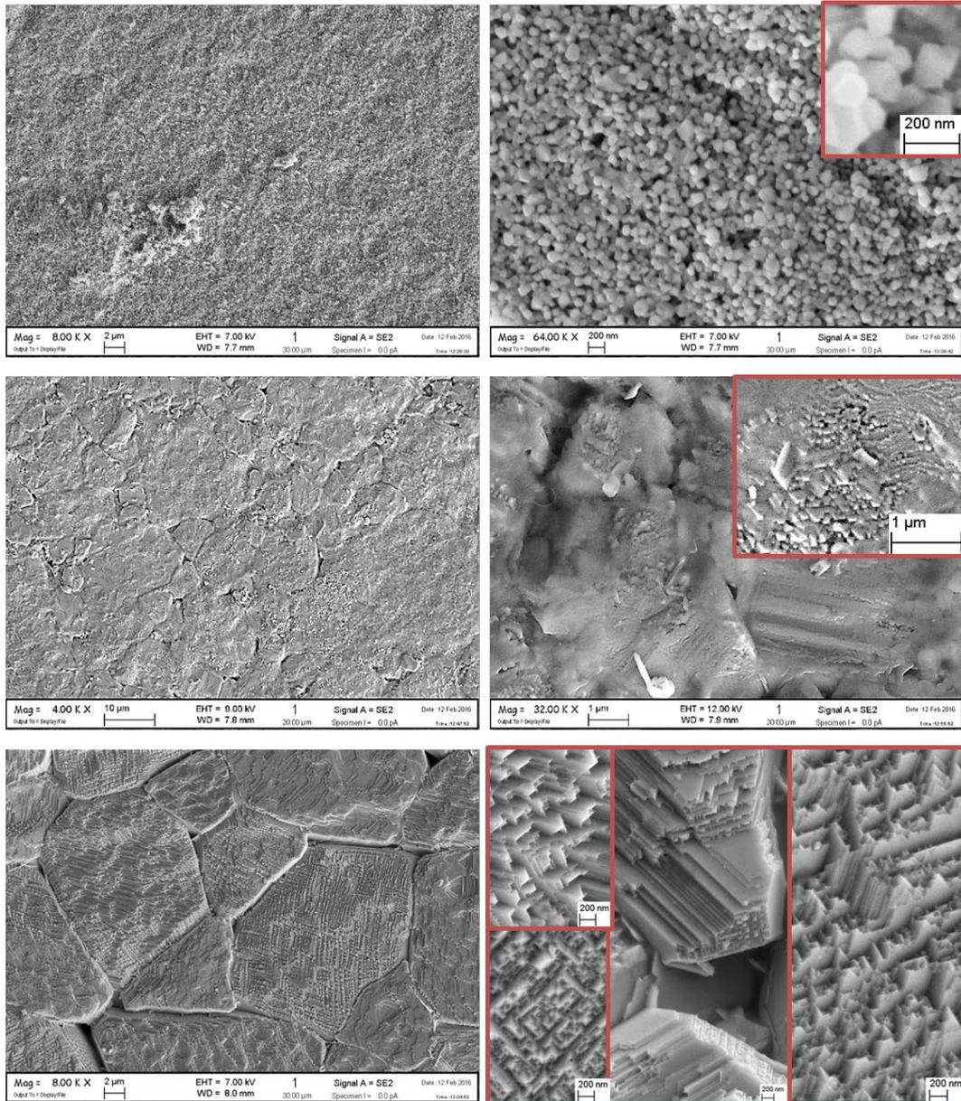
Fig. 3.12 SEM images of  $\text{CF}_{\text{sg}}7^1\text{-25}$  powders sintered by two-step sintering 830°C+780°Cx4h (first row); quite-fast sintering at 1250°C (second row); and conventional sintering at 1250°Cx2h (third row).
