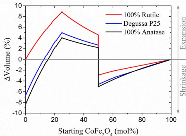
Fig. 3.25 Variations in volume predicted from the chemical reactions (Eq. 28) considering three different type of starting titania powders.
