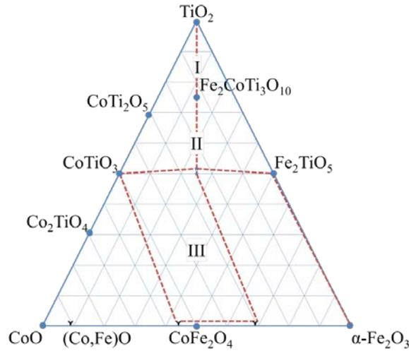
Fig. 3.23 Possible phase diagram of  $\text{CoO} - \text{TiO}_2 - \alpha\text{-Fe}_2\text{O}_3$  system at  $T = 1200\text{ }^\circ\text{C}$  and  $p(\text{O}_2) = 0.21\text{ atm}$ . The biphasic system of the triangle sides were drawn by starting from the Co-Ti-O [100], Fe-Ti-O [101], and Co-Fe-O (Fig. 3.1) systems.
