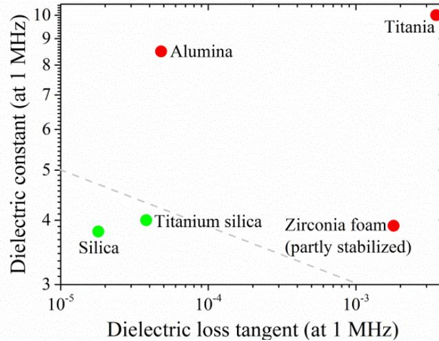
Fig. 3.27 Dielectric constant vs. dielectric loss tangent plot for alumina, silica, titania, and titanium silica (at 1 MHz). The values were taken from CES EduPack™ 2013 software's database.
