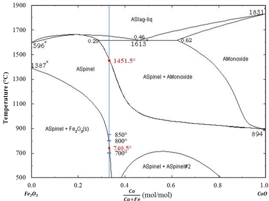
Fig. 3.1 Phase diagram of Fe – Co – O<sub>2</sub>, p(O<sub>2</sub>) = 0.21 atm, system.
