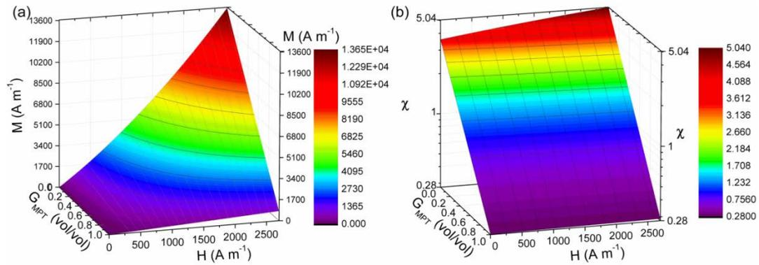
Fig. 3.16 (a) Magnetization and (b) susceptibility trend as a function of magnetic field strength ( $H$ ), and multiparallel-twinned grains volume fraction ( $G_{MPT}$ ) estimated through the mixing rule.
