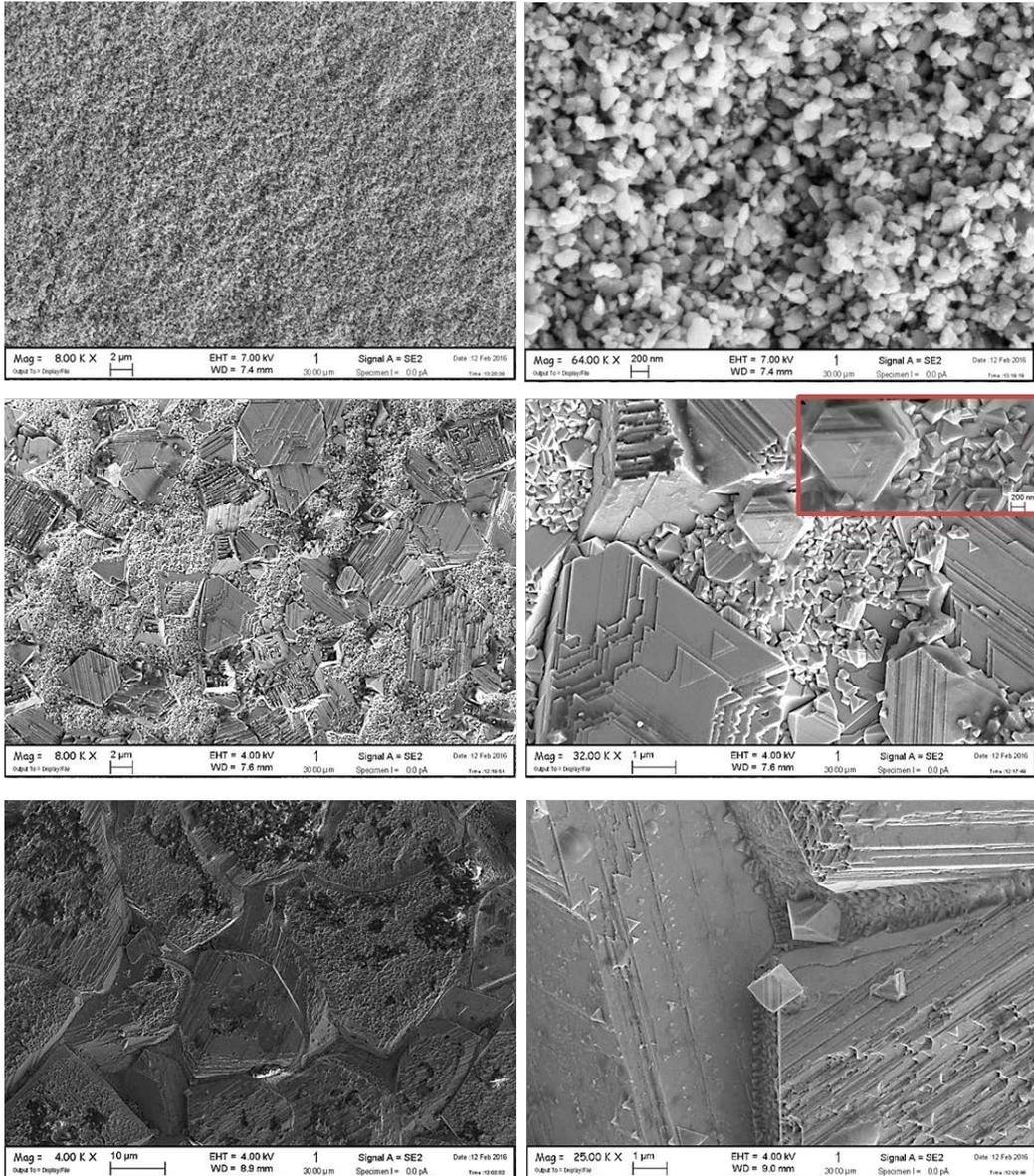
Fig. 3.13 SEM images of  $CF_{ss(n)}10^4-25$  powders sintered by two-step sintering 830°C+780°Cx4h (first row); quite-fast sintering at 1250°C (second row); and conventional sintering at 1250°Cx2h (third row).
