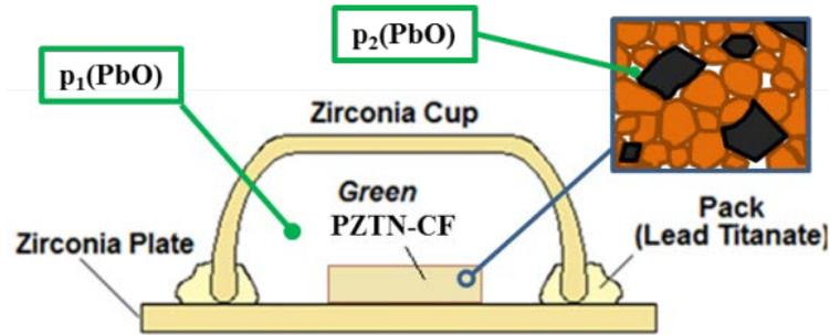
Fig. 3.31 Scheme of a green PZTN-CF sample surrounded by a mixture of PbO and  $PbTiO_3$  powders (also called atmosphere powder or pack), called pack, in order to provide a positive vapour pressure in a closed zirconia cup and contain the lead loss. However, inside the porosity of the sample lead activity,  $p_2(PbO)$ , is different from that outside the sample,  $p_1(PbO)$ . In the “zoom of microstructure” the orange grains and the black ones represent the PZTN and CF, respectively.
