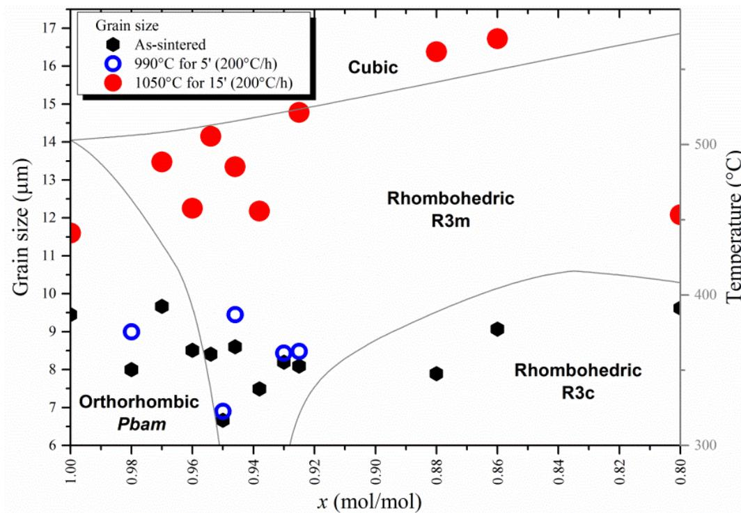
Fig. 3.21 (Left axis) Grain size vs. PZT composition,  $x$ , of as-sintered samples (black hexagons), and after heat treatment at 990 °C for 5 min (blue circumferences) and 1050 °C for 15 min (red circles). (Right axis) the corresponding phase diagram (grey lines).
