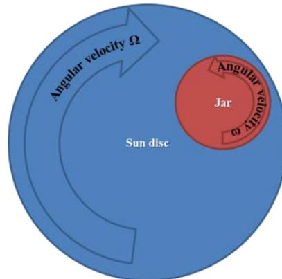
Fig. 2.10 Schematic draw of a planetary milling. For the Fritsch Pulverisette 6 (available at CNR-ISTEC), the effective diameter of main disk is 121.6 mm and transmission ratio planetary disk / grinding bowl is 1 : -1.82.
