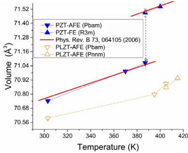
Fig. 2.24 Crystal volume of  $\text{PbZr}_{0.954}\text{Ti}_{0.046}\text{O}_3$  (PZT) and  $\text{Pb}_{0.97}\text{La}_{0.02}\text{Zr}_{0.954}\text{Ti}_{0.046}\text{O}_3$  (PLZT) vs. temperature [77]. FE and AFE refers to ferroelectric and antiferroelectric behaviour displayed by crystal lattice with R3m and Pbam symmetry, respectively.
