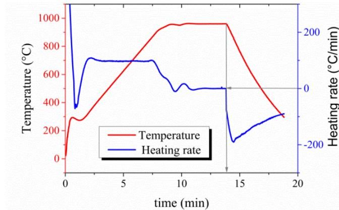
Fig. 3.7 Temperature and heating rate profiles collected by FCT/Germany SPS equipment and applying a pulsed current (on: 0.003 s; peak: 1600 A and 5 V). A pressure of 63 MPa was applied on the sample with thickness of about 2 mm and diameter of 20 mm.
