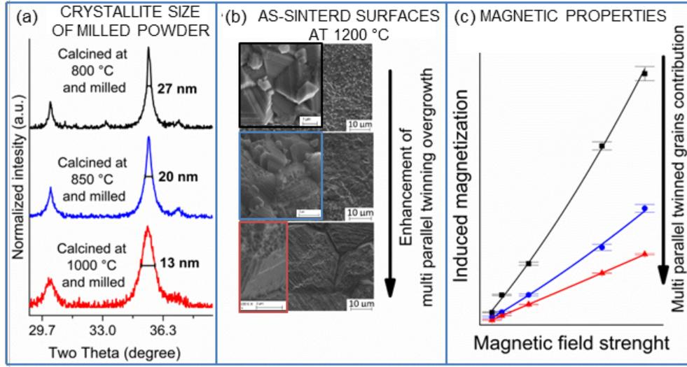
Fig. 2.9 Milling treatment effect on the crystal structure of CoFe<sub>2</sub>O<sub>4</sub> powders (a) and its knock-on effect of the microstructure evolution during the sintering process (b) and the correlation with the final magnetic properties (c).
