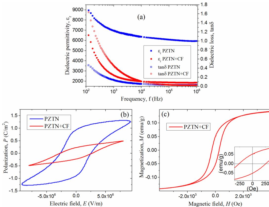
Fig. 3.39 (a) Dielectric permittivity ( $\epsilon_r$ ) and loss tangent ( $\tan\delta$ ) for the PZTN-cobalt ferrite bilayer vs. frequency. (b) and (c) electric and magnetic hysteresis loops, respectively, taken at room temperature.
