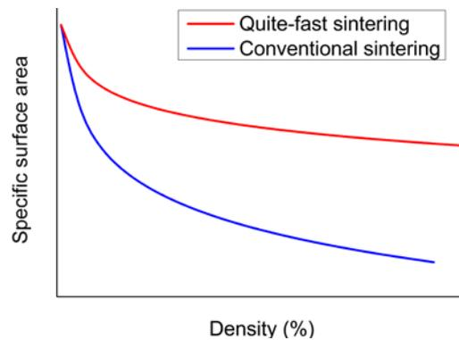
Fig. 2.20 Reduction of specific surface area vs. densification.
