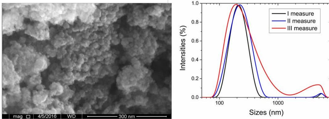
Fig. 2.27 SEM micrograph of planetary milled  $\text{CoFe}_2\text{O}_4$  and related dynamic light scattering analyses, separated by a gap of three minutes, of water suspension with 0.001 wt% of solid content.
