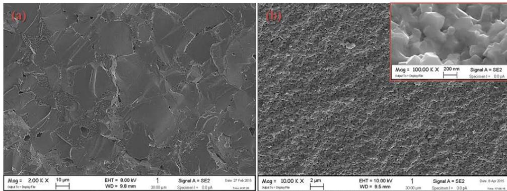
Fig. 2.18 Fracture surface of  $\text{CoFe}_2\text{O}_4$  sintered by (a) conventional sintering, and (b) quite-fast sintering. Their heating profile is that shown in Fig. 2.16.
