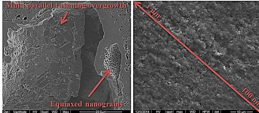
Fig. 3.8 Electron micrographs of a polished surface (left) and a fracture surface (right) of dense cobalt ferrite sintered by SPS at 950 °C for 5 min (Fig. 3.7) using  $CF_{sg}7^3$  powders (Fig. 2.4).
