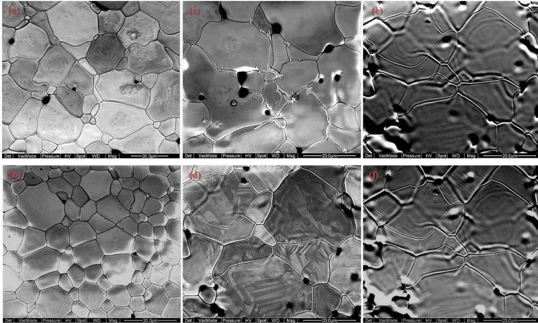
Fig. 3.22 Back-scattered electron micrographs of polished surfaces of PZT samples [(a, b)  $x = 0.8$ ; (c)  $x = 0.88$ ; (d-f)  $x = 1$ ] after thermal annealing at 1050 °C for 15 min. All bars are 20  $\mu\text{m}$ .
