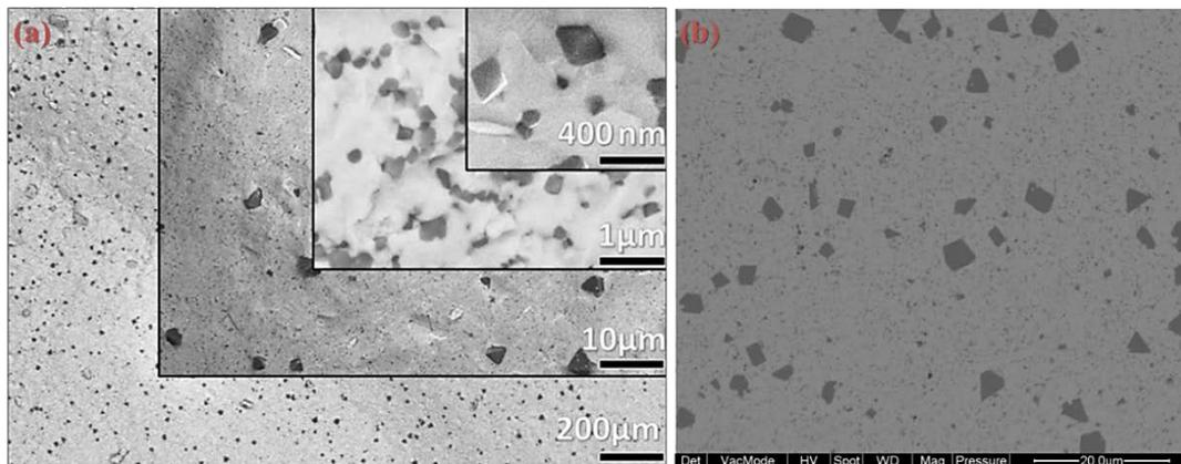
Fig. 3.37 (a) Back-scattered SEM images, at different magnifications, of fracture surfaces of sintered 0.87PZTN+0.13CF sample with bimodal size distribution of magnetic phase. (b) Its polished surface.
