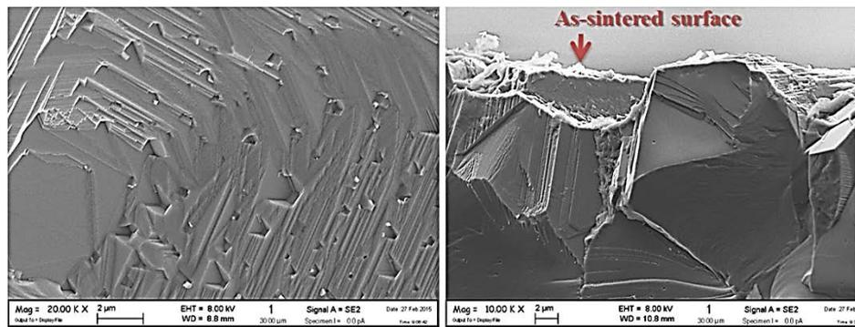
Fig. 3.17 SEM micrograph of fracture surface of cobalt ferrite sintered at 1200 °C for 2 h starting with  $CF_{10_{ss(n)}}^{4-25}$  powder.
