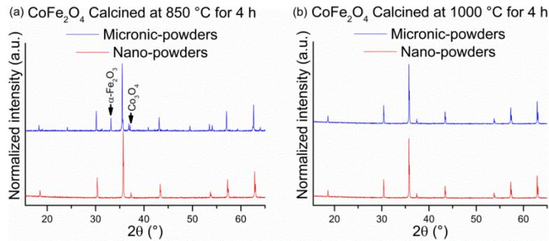
Fig. 2.1  $\text{CoFe}_2\text{O}_4$  powders synthesized starting from  $\text{Co}_3\text{O}_4$  and  $\text{Fe}_2\text{O}_3$  nanopowders (Aldrich 637025 and 544884, respectively) or micropowders (Alfa Aesar 45806 and Aldrich 310050, respectively) and calcined at (a) 850 °C for 4 h and (b) 1000 °C for 4 h.
