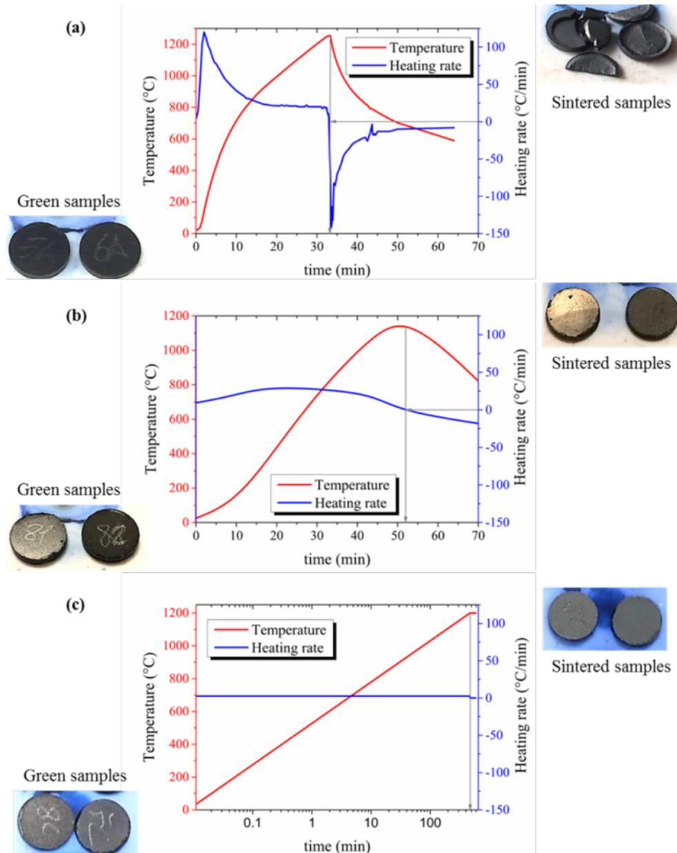
Fig. 3.6 (a and b) quite-fast sintering and (c) conventional sintering of  $\text{CF}_{\text{ss}(\mu)}85^{4+8}-40$  and  $\text{CF}_{\text{ss}(\mu)}105^4-40$  powders.
