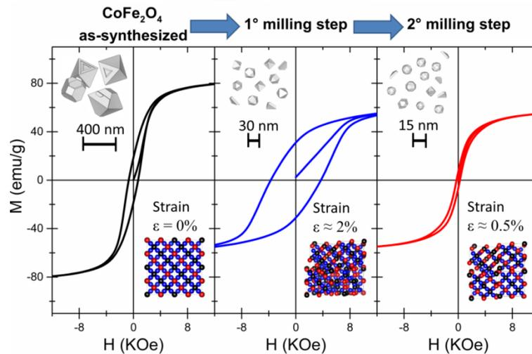
Fig. 2.8 Magnetization vs. magnetic field strength plots of as-calcined  $\text{CoFe}_2\text{O}_4$  and the milled one and two times. The particle size and the microstrain of each step (calculated through Rietveld analysis) is shown, since these two parameters have a considerable weight on the magnetic hysteresis shape.
