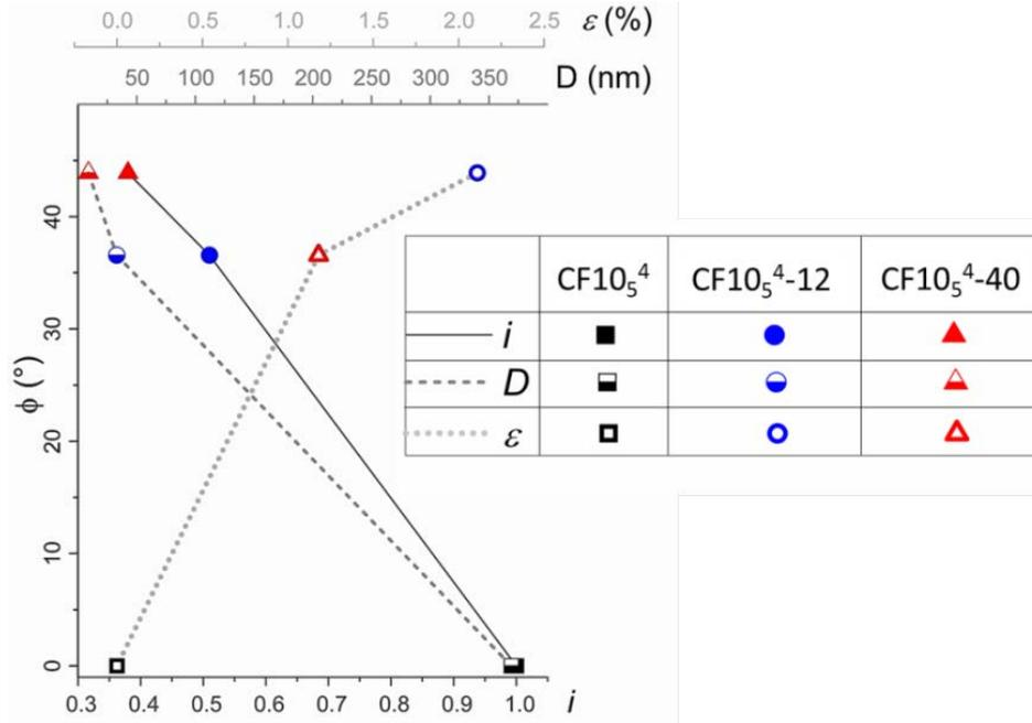
Fig. 3.5 The variation of spin-canting angle  $\phi$  with  $i$  (solid line); and the variation of  $\phi$  angle as function of the measured crystallite sizes and strains (dashed line with half-open and open symbols, respectively).
