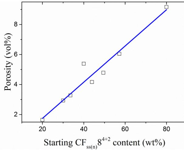
Fig. 3.26 Porosity vs.  $\text{CF}_{\text{ss(n)}}\text{8}^{4+2}$  content in starting powder mixtures
