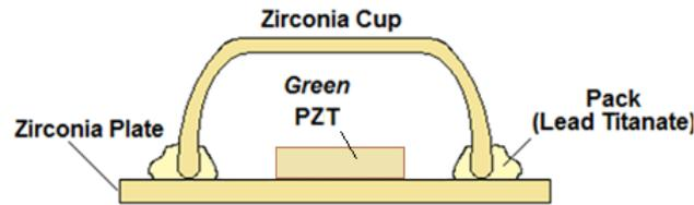
Fig. 2.17 Scheme of a green sample of lead zirconate titanate (PZT) surrounded by lead-based powders, called pack (a mixture of  $\text{PbO}$  and  $\text{ZrO}_2$  or  $\text{PbTiO}_3$  powders), in order to provide a positive vapor pressure in a closed zirconia cup and contain the lead loss. Similar scheme, but with different composition pack, can be used to prevent the loss of other volatile elements such as Na, Bi, etc.
