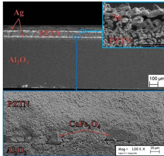
Fig. 3.38 Backscattered electron micrograph of fracture surface of magnetolectric layered composite. All the insets are secondary electron micrograph.
