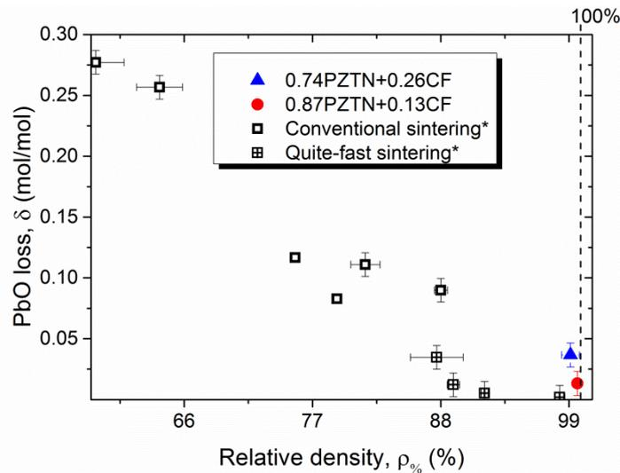
Fig. 3.33 PbO loss of 0.74PZTN-0.26CF (triangle), 0.87PZTN+0.13CF (circle), and PZTN+CF composites reported in (\*) Ref. [19] (square symbols) vs. their relative density.
