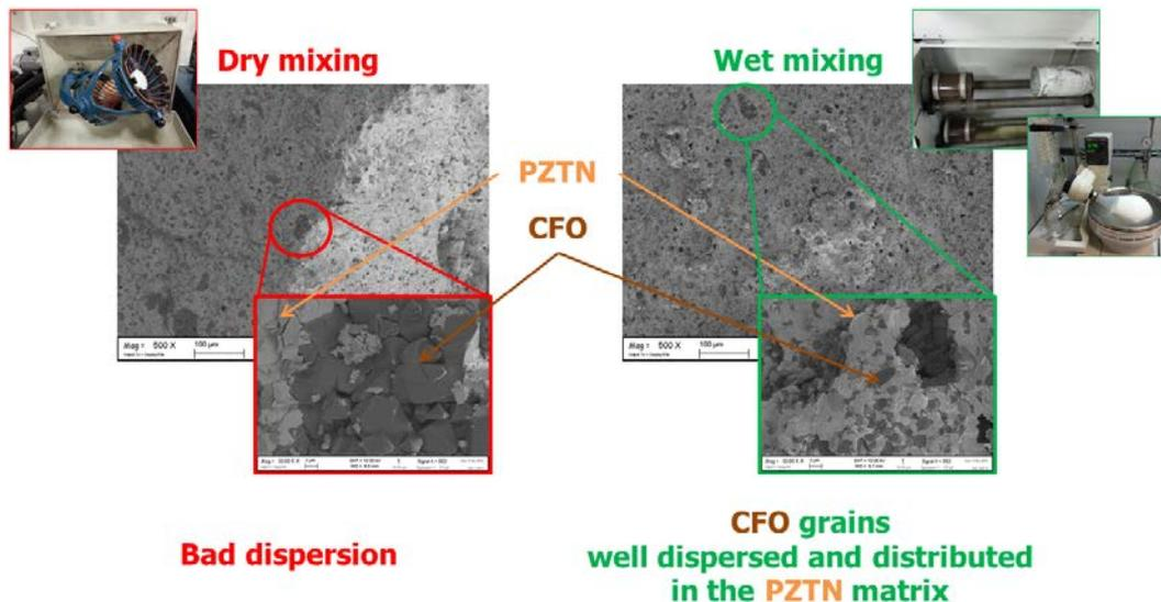
Fig. 2.14 Comparison of dry/wet mixing influence on the sintered microstructure of  $(1-x)\text{Nb}$ -doped lead zirconate titanate (PZTN) –  $(x)$ cobalt ferrite (CFO) composite, with  $x = 26 \text{ mol}\%$ .
