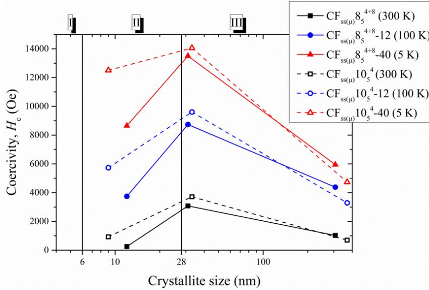
Fig. 3.3  $H_c$  dependence on crystallite size at various temperatures for:  $CF_{ss(\mu)}8_5^{4+8}$  series (solid lines) and  $CF_{ss(\mu)}10_5^4$  series (dashed lines). The superparamagnetic region, the single domain region, and the multi-domain region are labeled with I, II, and III, respectively.
