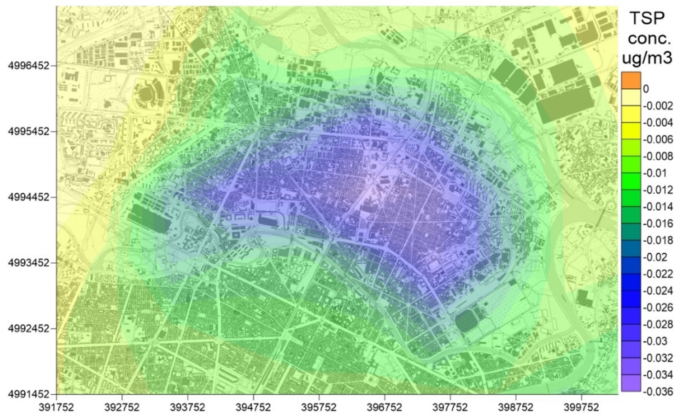
Figure 3.40. Map of TSP concentration difference at ground level in the urban area of Turin, month of January, simulating residential emissions as areas sources (zoom to the areas interested by the DH network extension).
