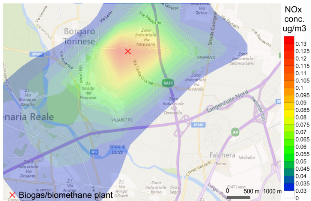
Figure 2.19. NO x concentration map at ground level (modeled with CALPUFF) generated by the biogas combustion plant (Scenario 3-B, future situation).
