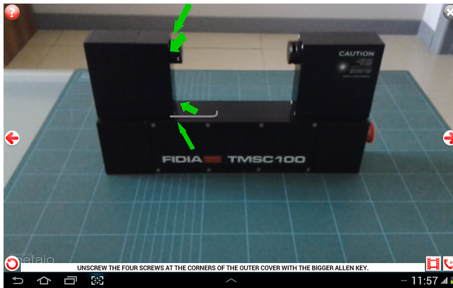
Fig. 1.3 AR application for maintenance procedures. The application supports the technician through the repair task of an industrial device; textual and 3D assets are shown.
