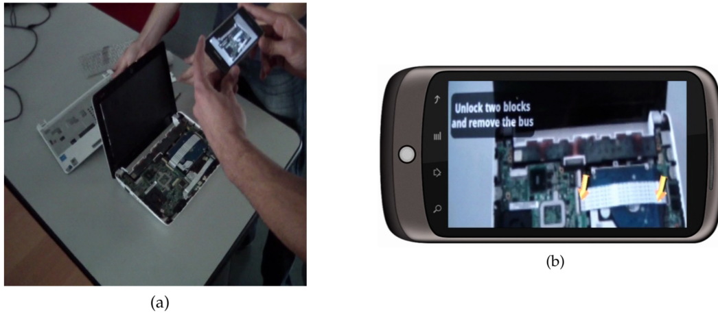
Fig. 2.2 Handheld Augmented Reality for maintenance operations: a) real object under maintenance framed by a smartphone, b) close look on the HAR application graphics interface.
