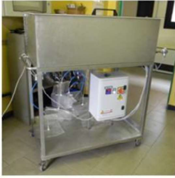
Figure 1. Apparatus for anaerobic digestion tests
