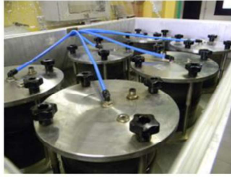
Figure 1. Apparatus for anaerobic digestion tests
