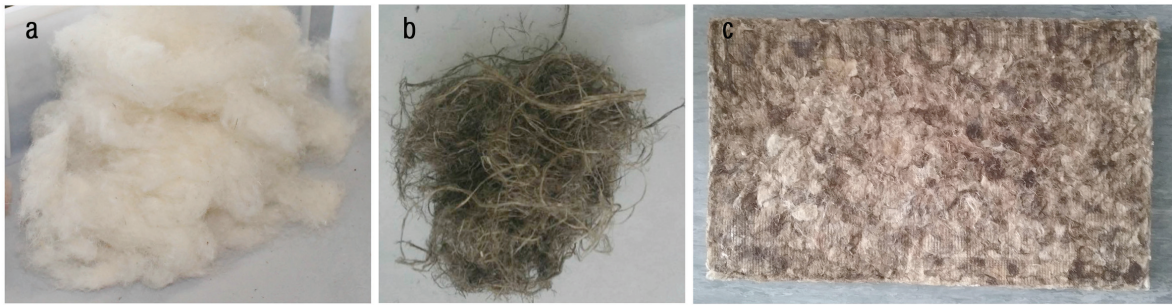
Fig. 1. a) Washed wool fleece, b) Hemp fibres retted in field, c) FITNESs panel
