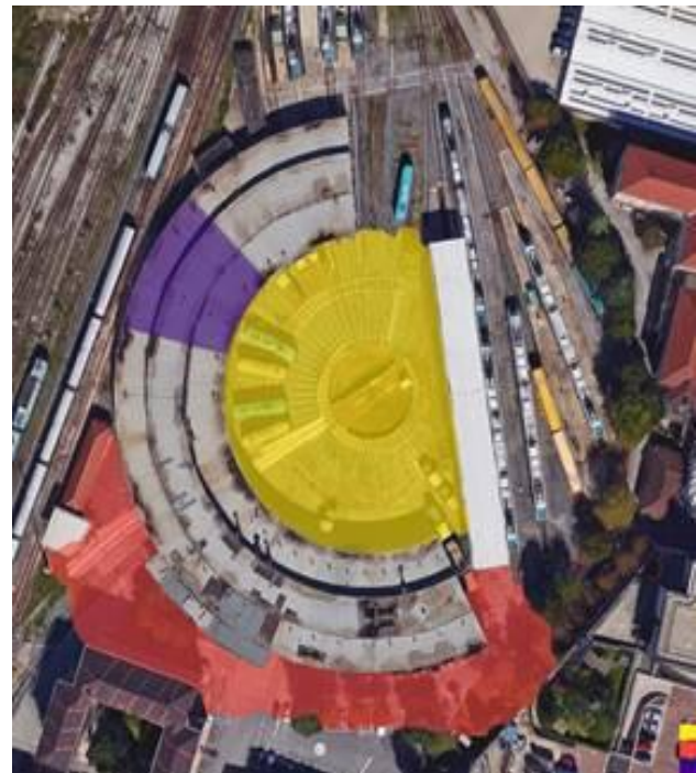
Figure 4. The thematic subdivision of the surveyed areas: in purple internal survey (TLS), in yellow external courtyard (TLS and SfM); in red topographic survey.
