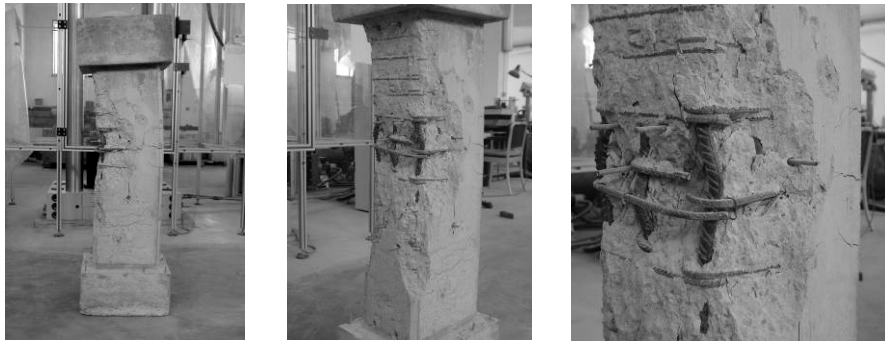
Figure 4.4. Specimen CEY2 after test
