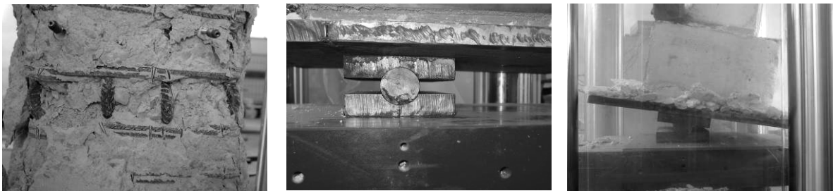
Figure 4.6. Ultimate state of specimen CEX1; rotation of device at the top and base of specimens
