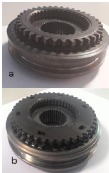
Figure 4. (a) single cone and (b) double cone synchronizers used for testing.
