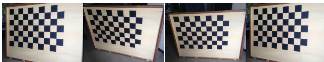
Figure 11. Some images of the checkerboard acquired by a smartphone for camera calibration.
