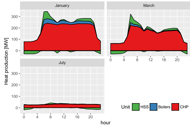
Figure 5: Average heat load for some months (heating seasons from 2007/2008 to 2010/2011).
