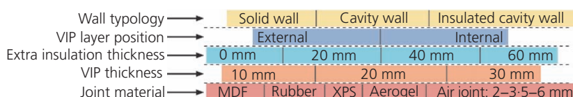
Figure 3. Different combinations of wall configurations
