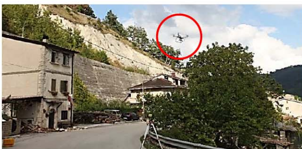
Figure 6. Phantom 4 DJI piloted drone (in red circle) during aerial acquisition
