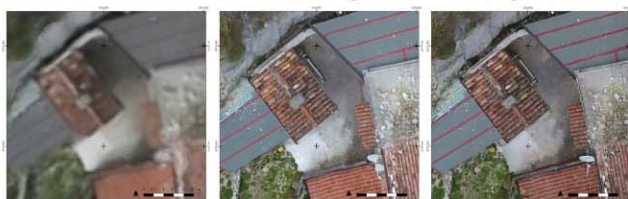
Figure 12. Comparison for a zoomed excerpt: eBee, average GSD=5 cm/px (left); DJI Phantom, average GSD=2,18 cm/px (centre); fusion model, average GSD=0.92 cm/px (right)
