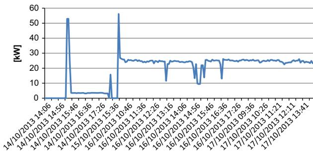
Fig. 3. Power profile of the crusher F1.
