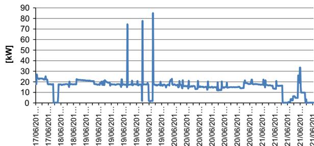
Fig. 2. Power profile of low temperature seed micronizer.
