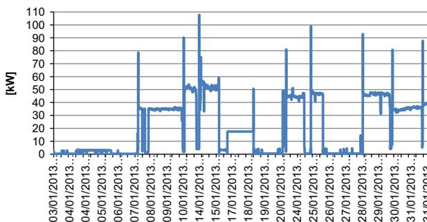
Fig. 4. Power profile of the crusher F2.
