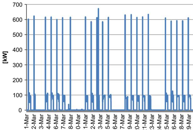
Fig. 1. Power profile of the corncob crusher.
