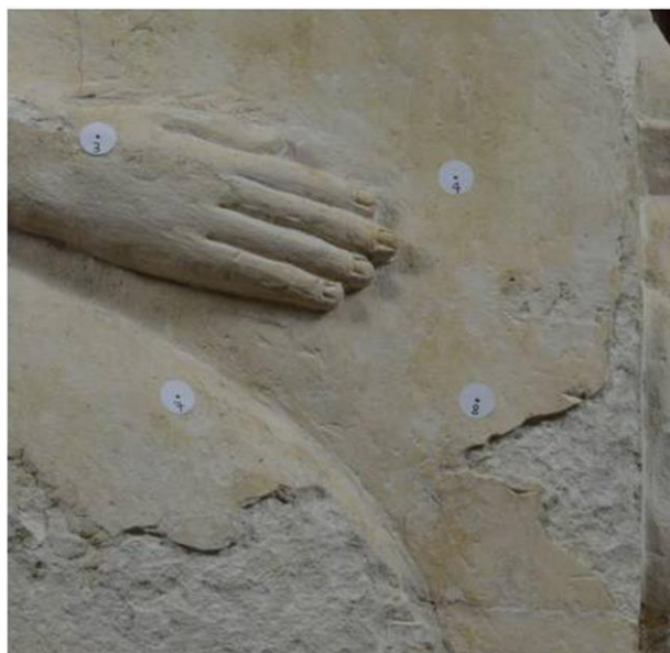
Figure 8. Some circular sticky stamps used to materialize TX and RX points.
