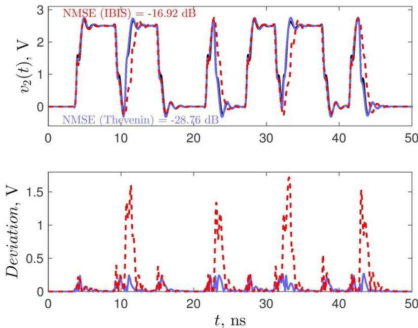
**Fig. 7.** Output port voltage response of the example buffer loading an transmission line with 60 Ohm characteristic impedance, 0.1 ns delay and a far end 7 pF capacitor. Solid black: reference response; solid blue: Thevenin model prediction; dashed red: IBIS model prediction.
