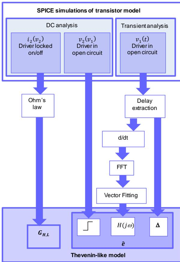
Fig. 6. Flow chart illustrating the algorithm described in section 3.
