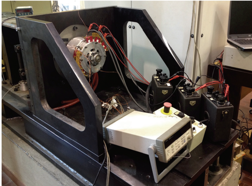
Fig. 6.2.5. Prototype mounted on the test bench for the thermal tests.
