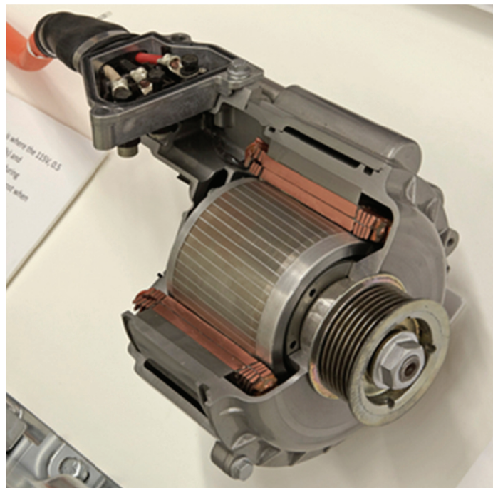
Fig. 3.3.4. GM e-assist belt alternator starter, BAS [32].
