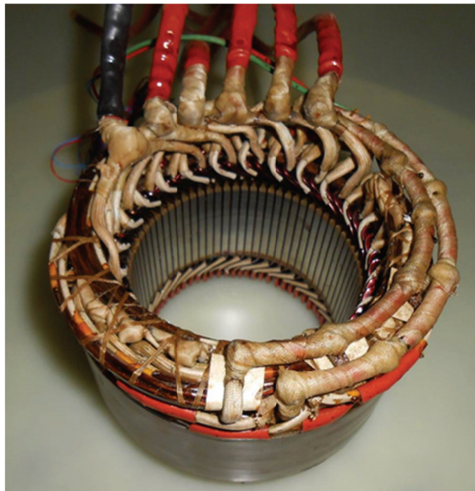
Fig. 4.2.2.5. Detail of the stator end-turn connections.
