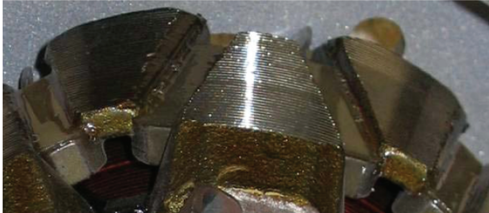
Fig. 3.3.1 Claw-pole machine: magnets inserted between the pole [11]
