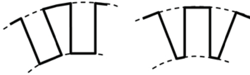
Fig. 4.2. Rectangular slot (a) and trapezoidal slot(b)
