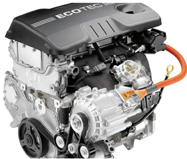
Fig. 2.3.4. GM Belt-Alternator Starter mild-hybrid drivetrain [19].
