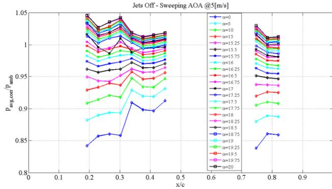
Figure 13 - Mean pressure chord-wise distribution sweeping AOA
