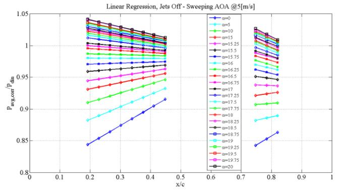
Figure 14 - Linearized mean pressure chord-wise distribution sweeping AOA
