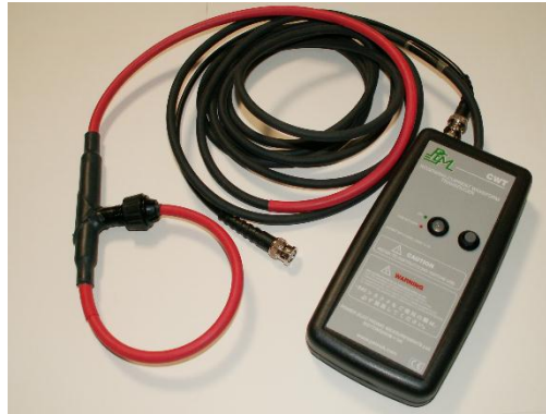
Figure 3. The electrical transducer (Rogowski coil and integrator device) used in the welding tests [14].
