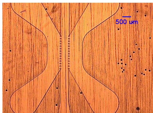
(B) SU8 pattern on a polished Cu plate
