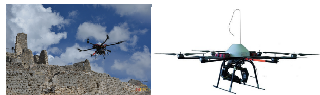
Figure 2. The employed platform - UBIK DIATI MK01
