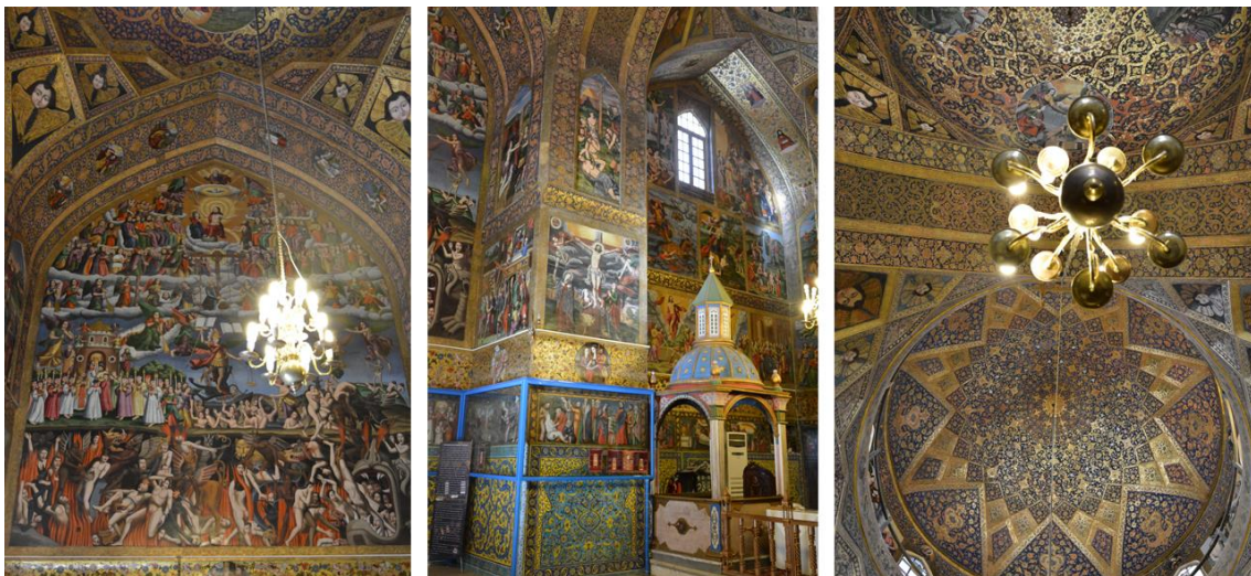
Figure 2. The beautiful frescoed walls of the Vank cathedral with the highlights of some critical elements for photogrammetric processing: the presence of chandeliers and transparent protections at visitors' heights.
