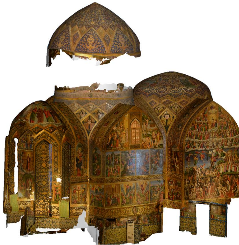
Figure 5. The entire meshed model with high-resolution textures representing frescoes; the lack of surface above the drum of the dome is obvious due to the impossibility to take pictures.
